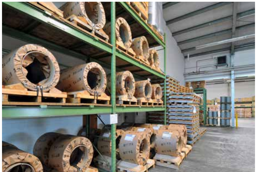
Storage of coils with wooden sleepers
